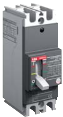
A1 100A TMF - Fixed (F) - 2 pole - Front terminals (F) - UL/CSA - Thermal-Magnetic (TMF) 240Vac
